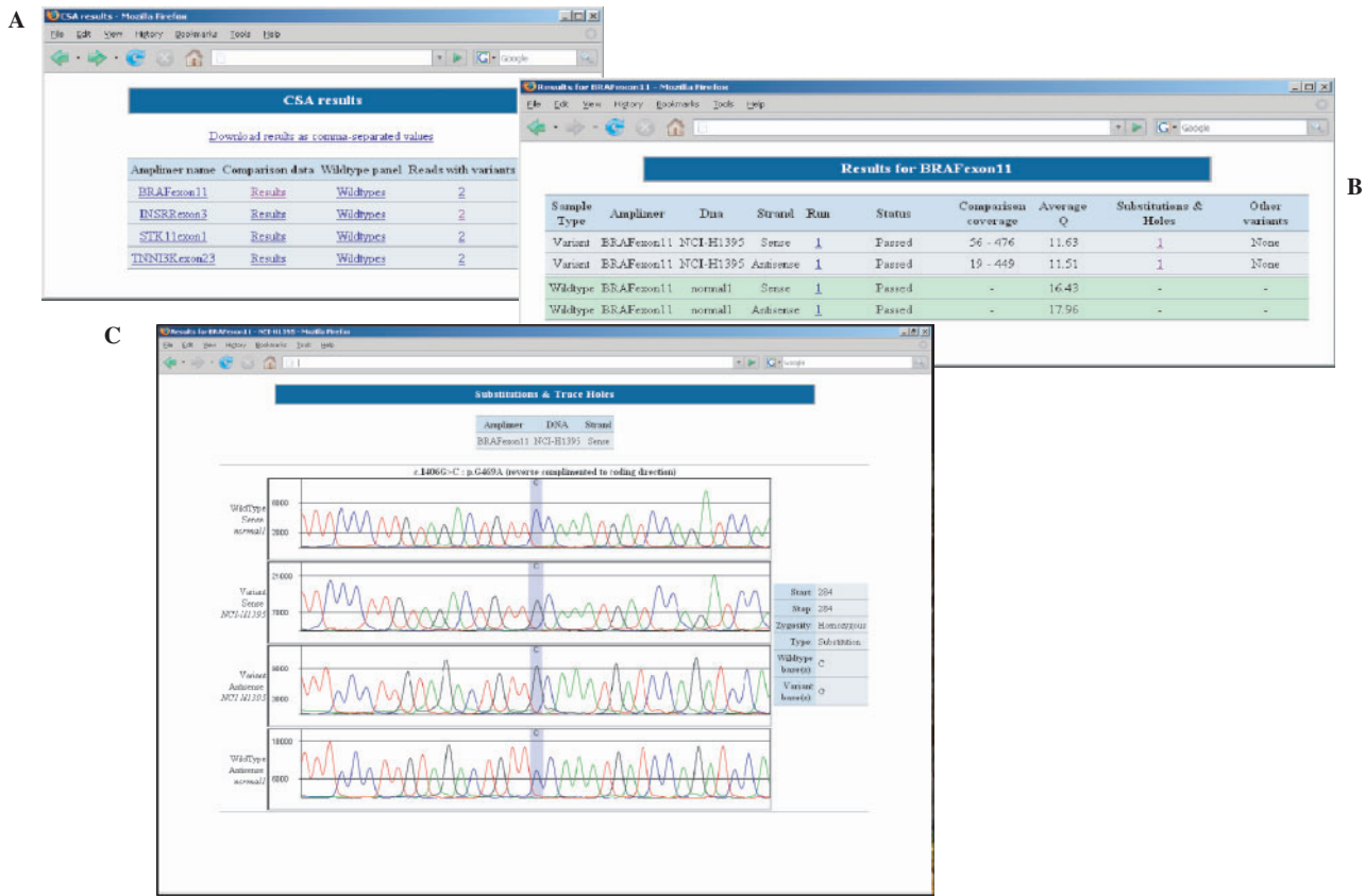
Fig. 1. AutoCSA displays (A) Lists all sequences screened with a summary of variants found. (B) Lists traces screened with coverage information and number of variants on each trace. (C) Main substitution display, four traces are displayed with 20 bases either side of the potential substitution. The top two traces are the traces which were used to call the variant (reference first and trace under investigation second). The third and fourth traces are the reverse sequenced traces. The DNA and protein annotation of the variant are displayed above and to the right of the traces.
